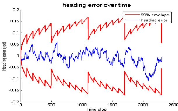
Fig. 2. 99% envelope computed by the filter for the heading error (red line), and the true heading error (blue line). The variance is reduced at each relative displacement observation but overall grows until landmarks with known locations are observed.
