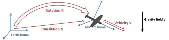
We consider here the more complicated model of an UAV evolving in the 3D space and whose state is parameterized by its attitude  $R_t$ , velocity  $v_t$  and position  $x_t$ . The vehicle is equipped with an IMU (accelerometers and gyroscopes) whose measurements are denoted respectively by  $u_t$  and  $\omega_t$ . The continuous time dynamics read:
