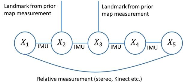
Fig. 1. Factor graph representation of the measurements relating the states (nodes). The IMU measurements relate any two consecutive states, whereas from time to time landmarks with known locations are observed, and matching images obtained at different time instants allows to relate some non-consecutive states.
