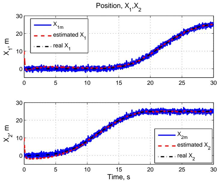
**Figure 5.** Estimated, true, measured position,  $X_1, X_2$  (simulation)
