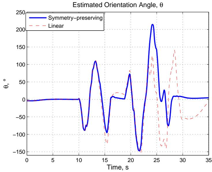
**Figure 7.** Orientation angle estimation (experiment)
