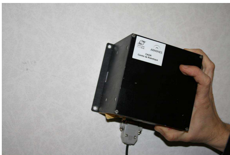
Figure 6. Experimental setup : inertial measurement unit on a wall
