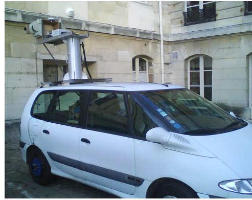
Fig. 3. Used vehicle and IMU/GPS on the roof
