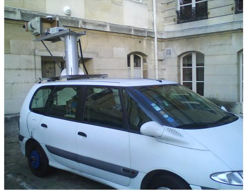
Fig. 3. Used vehicle and IMU/GPS on the roof
