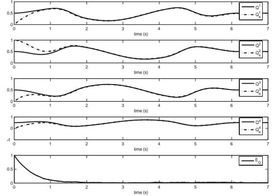
Fig. 3. Idem: four coordinates of attitude  $q$  (solid line) and estimated attitude  $\hat{q}$  (dashed-line); estimation error  $E_Q = \|q^{-1}\hat{q} - 1\|$  using left-invariant EKF (20). The only difference with Fig 2 is that the initial condition  $q(0) = [0.5, 0.5, 0.5, 0.5]$  is different, but  $\eta(0)$  is the same. Although the trajectory  $q(t)$  is different, the error  $E_Q$  has the same behavior.
