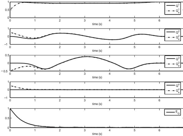
Fig. 2. Four coordinates of attitude  $q$  (solid line) and estimated attitude  $\hat{q}$  (dashed-line); estimation error  $E_Q = \|q^{-1}\hat{q} - 1\|$  using left-invariant EKF (20).
