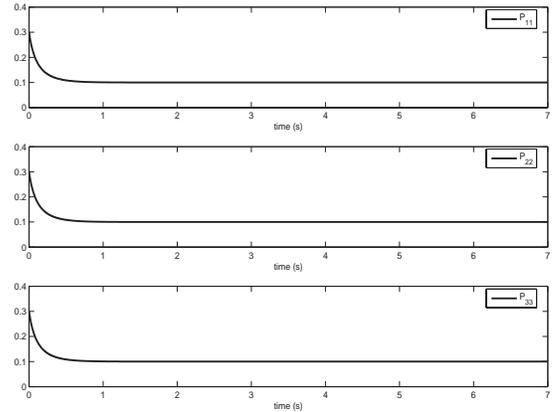
Fig. 4. Diagonal coefficients of the matrix  $P$ . Every parameter is the same as in section V except that here we took  $P(0) = 0.3 * I_3$  to illustrate the convergence of the diagonal coefficients.
