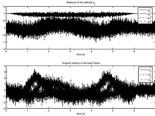
Fig. 1. Measured noisy signals : attitude  $q_y$  and angular velocity  $\omega$  (rad/s) in the body frame.
